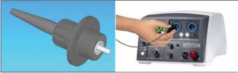
Figure 3. ENGAUGE RFID automatically recognizes the type of device being connected. Laser settings can be preset and automatically loaded when the type of delivery device is identified.
